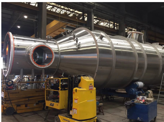
Figure 2. Crystalliser manufactured using VDM Alloy 31 Plus. The manufacturing process took place at ZIEMEX.
