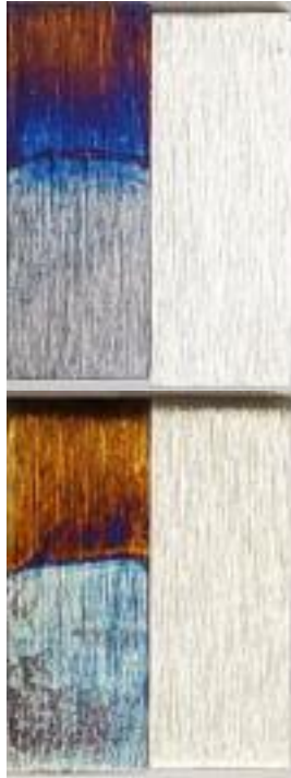
Figure 2: The alloy samples are shown after and before testing from left to right with UNS N06230 above and UNS N06625GR1 below.
