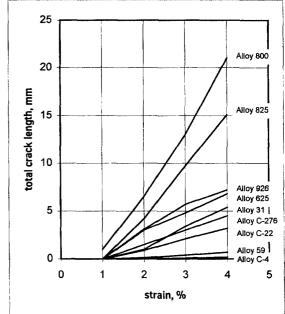
Figure 2: Modified Varestraint-Test (MVT) for the Evaluation of the Hot Cracking behaviour <sup>(16)</sup>
