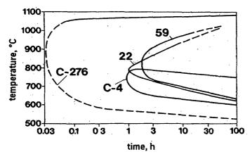
Figure 1: Time-Temperature-Sensitization Diagram of several Ni-Cr-Mo Alloys (13)
