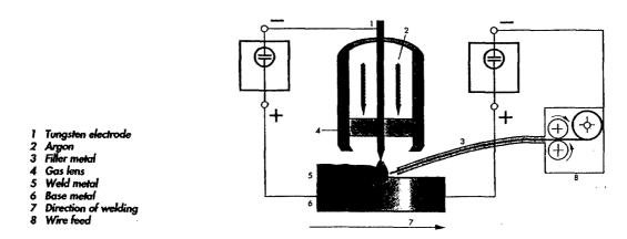
Figure 4: Gas Tungsten-Arc Hot Wire Welding (GTAW-HW)
