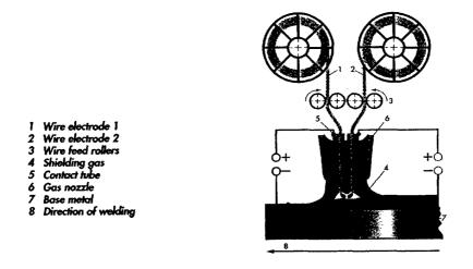
Figure 5: Metal Active Gas Tandem Welding (MAG Tandem Welding)
