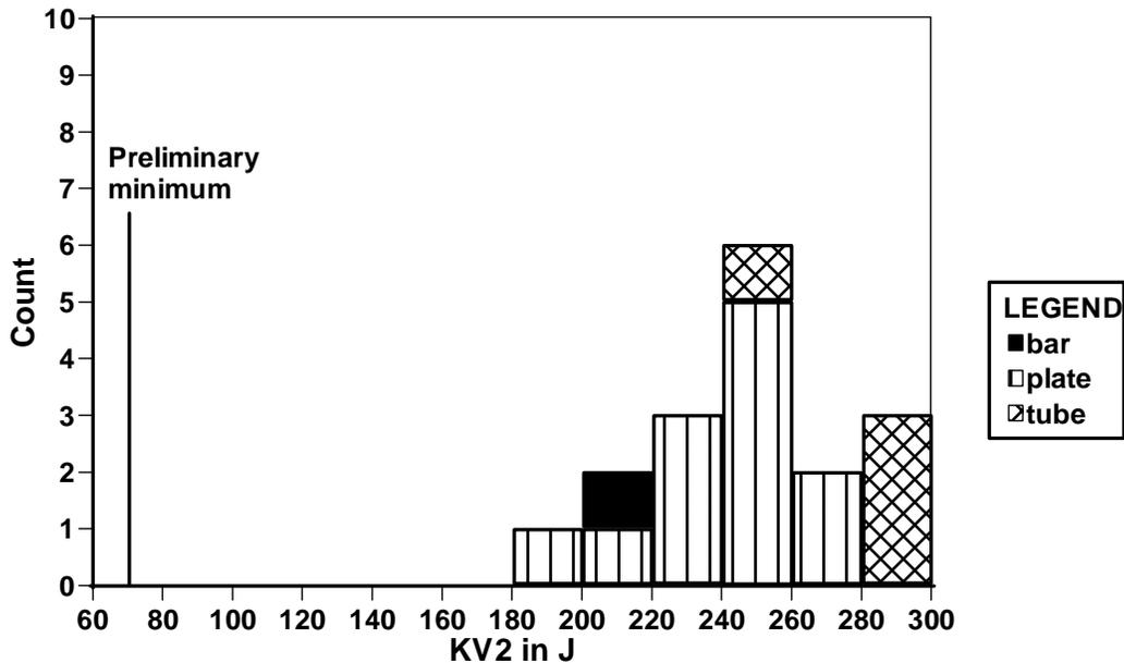
**Figure 6: Histogram of the V-notch bar impact energy KV<sub>2</sub> at room temperature on alloy 699 XA bar, plate and tube.**
