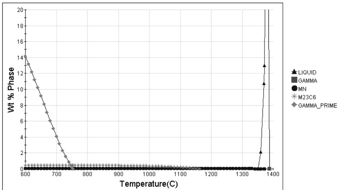
Figure 3: Phase diagram of alloy 699 XA calculated with JMatPro V9.0
