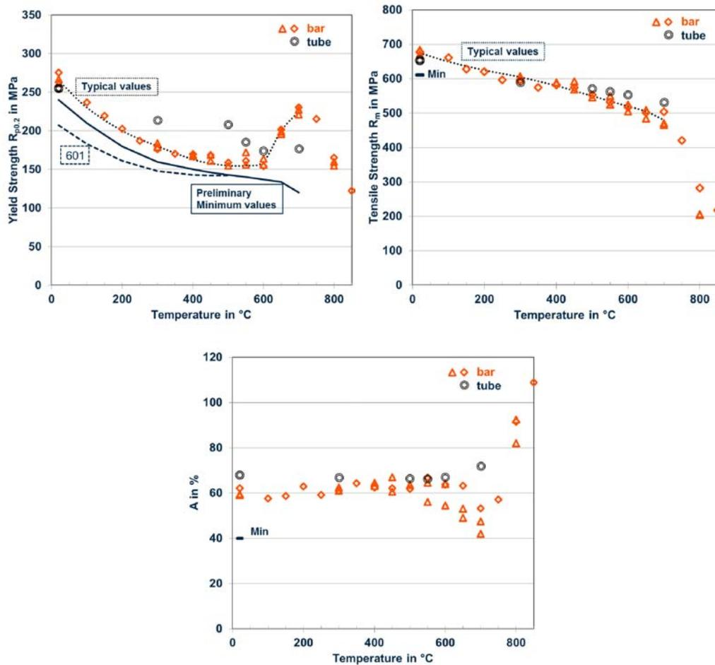
**Figure 5: Yield and tensile strength and elongation of hot tensile tests on alloy 699 XA bar and tube (solution annealed), triangle measured by <sup>40</sup>**
