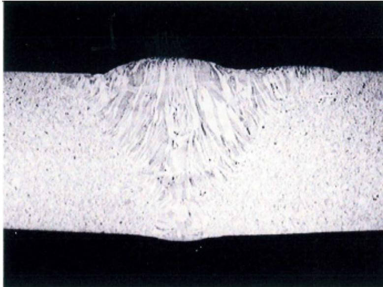
**Figure 8: Macroscopic picture of the weld<sup>57</sup>**
