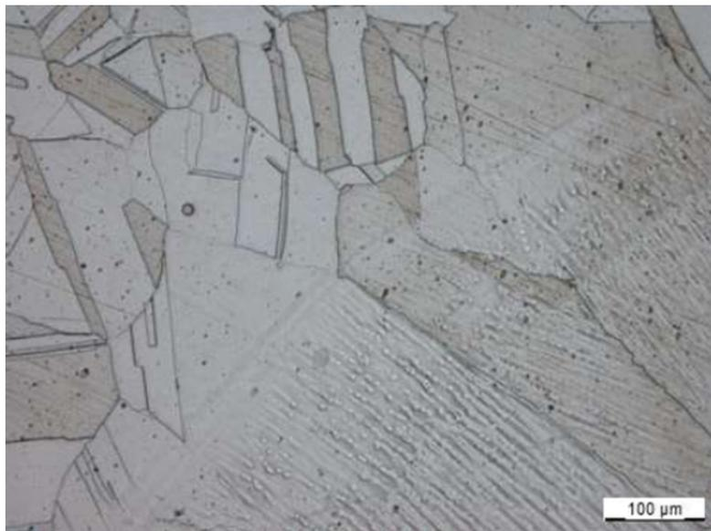
**Figure 9: Metallographic picture of the weld and the heat affected zone.**
