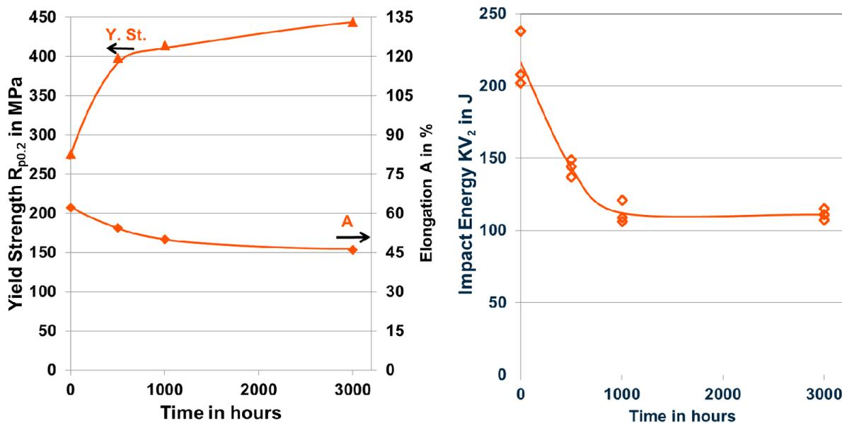
**Figure 7: Yield strength and elongation (left) and Charpy V-notch impact energy after annealing solution annealed samples of alloy 699 XA, heat 318385 - bar up to 3000 h at 600°C.**
