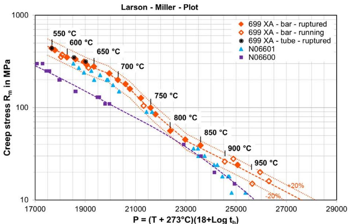
**Figure 4: Larson-Miller-Plot of the creep results of alloy 699 XA on bar<sup>40, 41</sup>, alloy 699 XA on tube, N06600<sup>42, 43</sup> and N06601<sup>44-50</sup> T: test temperature in °C,  $t_b$ : time to rupture in hours.**
