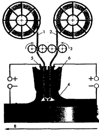
Figure 5: Metal Active Gas Tandem Welding (MAG Tandem Welding)
