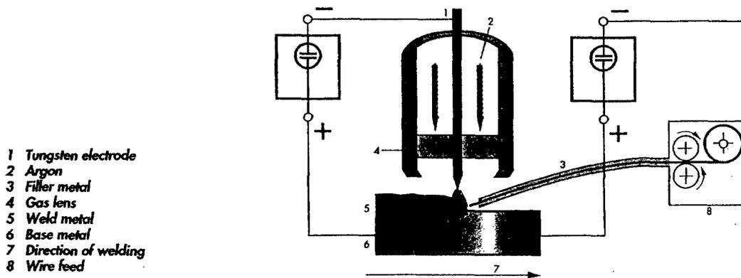
Figure 4: Gas Tungsten-Arc Hot Wire Welding (GTAW-HW)
