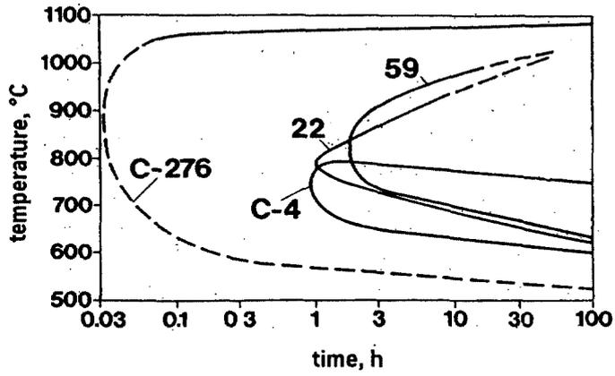
Figure 1: Time-Temperature-Sensitization Diagram of several Ni-Cr-Mo Alloys <sup>(13)</sup>
