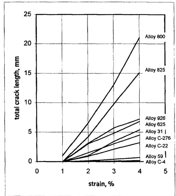
Figure 3: Hot Cracking Behaviour of different Ni-Cr-Mo Alloys
