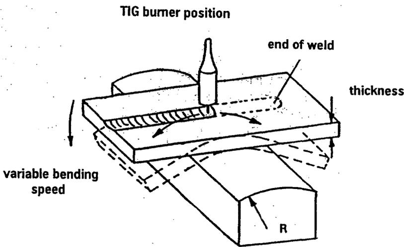
Figure 2: Modified Varestraint-Test (MVT) for the Evaluation of the Hot Cracking behaviour <sup>(16)</sup>
