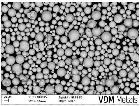
The picture shows a typical micrograph of VDM® Powder X as an example.
