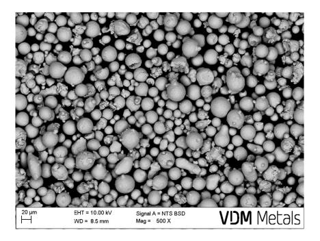
The picture shows a typical micrograph of VDM® Powder CoCr F75 as an example.
