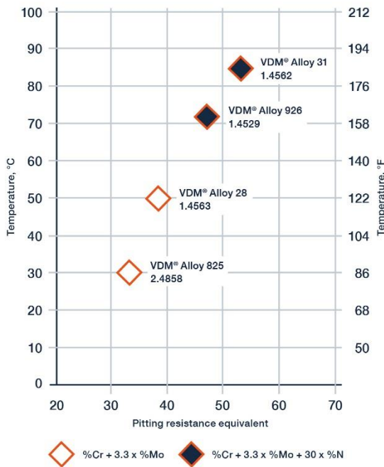
Fig. 1 – Critical pitting corrosion temperature in 10 % FeCl3 x6H2O solution as a function of the effective sum in comparison to some stainless steels and nickel alloys.
