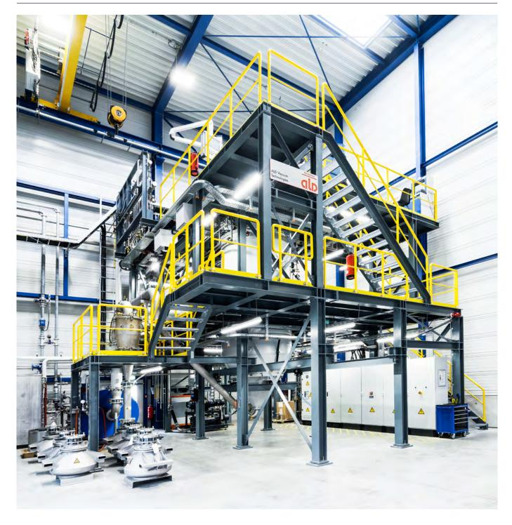
the powder collecting tank. In the plant the high-purity powder is produced by means of vacuum induction melting and inert gas atomization. The individual steps of the powder production are precisely coordinated to each other, as they affect the composition and purity of the powder. The entire process occurs in vacuum and inert gas conditions, so as to ensure as high a purity as possible.
