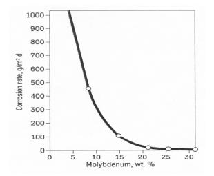
**Fig. 4:** Corrosion rate of binary nickel-molybdenum alloys in boiling 10 % hydrochloric acid as function of the molybdenum content (from K. E. Volk, 1970 [7])
