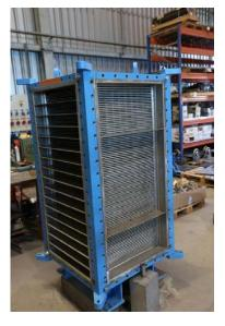
**Fig. 9**: Application of alloy UNS N06058 as material of construction for: (left side) heat recovery systems for indirect heat transfer in a FGD plant and (right side) plate heat exchangers for hydrochloric acid in a chemical plant (equipment manufactured by ZIEMEX).
