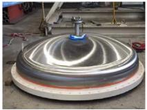
**Figure 12:** Example of application of alloy UNS N08034 for evaporators in the salt industry. Equipment manufactured by ZIEMEX.
