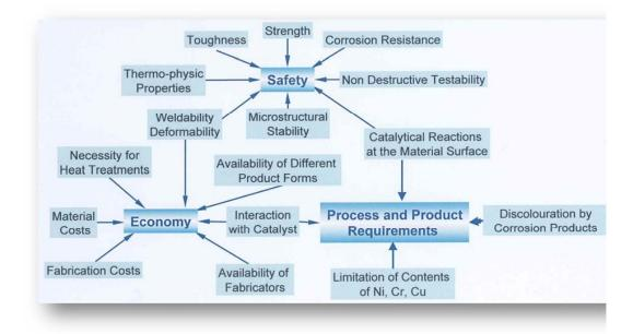
Fig. 1: Criteria for material selection in the process industry (from J. Korkhaus, ACHEMA 2006 [1]).
