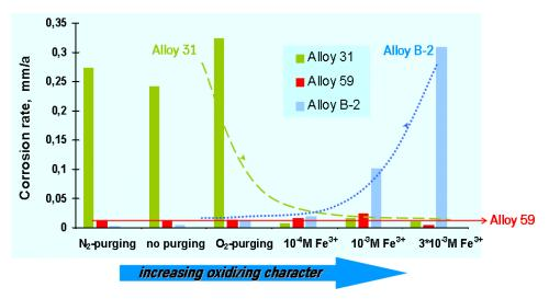
**Fig. 13:** Corrosion behaviour of a nickel-chromium-molybdenum alloy (alloy 59), a nickelchromium-iron-molybdenum-copper alloy (alloy 31) and a nickel-molybdenum alloy (alloy B-2) in an aquous solution with increasing oxidizing character
