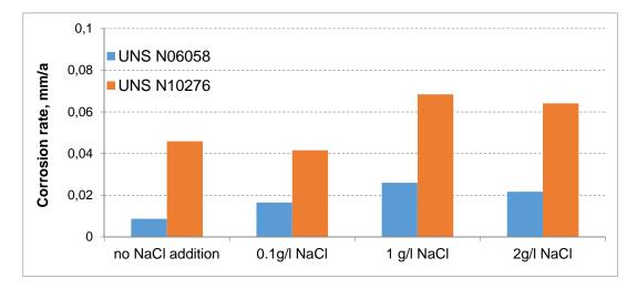
**Fig. 8:** Corrosion rate (mm/a) of alloy UNS N06058 test samples in 50 % acetic acid + 40 % formic acid + 5 % sulphuric acid at 95 % without and with different additions of chlorides in form of NaCl in comparison to alloy UNS N10276. Testing period for immersion 24 hrs.
