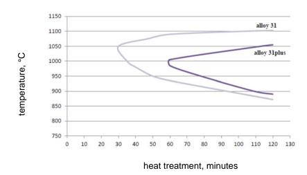
**Fig. 11:** Diagram representing the lines where the ISO V-notch impact strength decreases from initially more than 250J to a value of 50J as a function of the heat treatment temperature and time for alloy UNS N08034 and alloy UNS N08031. Testing done at - 60 °C.
