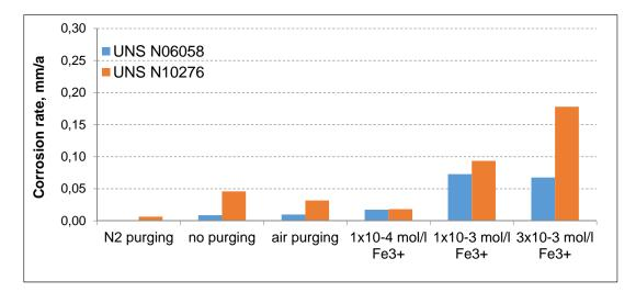
**Fig. 7:** Corrosion rate (mm/a) of alloy UNS N06058 test samples in 50 % acetic acid + 40 % formic acid +5 % sulphuric acid at 95 °C under different oxidizing conditions in comparison to alloy UNS N10276. Testing period for immersion 24 hrs.
