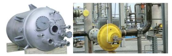
**Fig. 6:** Application of alloy UNS N06059 as material of construction for: (left side) reactor for the production of catalysts and (right side) piping for a HP-technology melamine plant.
