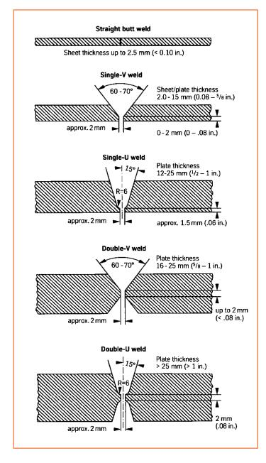
Figure 1 – Seam preparation for welding nickel alloys and special stainless steels
